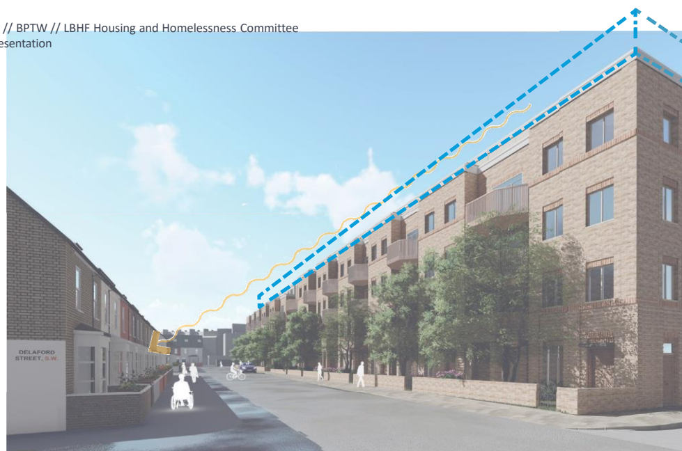
Balancing sustainability principles and design considerations: The fifth storey on Pellant Road is set back to create a better balanced relationship with the existing houses
